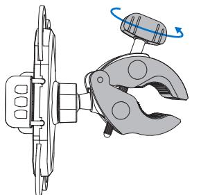
5. Install the bicycle fixed clip on the bicycle handle, and tighten the adjusting screw to fix the bracket.
