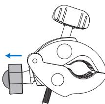
3. Align the round hole on the back of the phone clip with the connecting ball and push firmly, and tighten the fixed nut.
