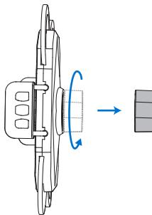
2. Put the fixed nut on the connecting ball of the bicycle fixed clip (the connecting ball must face the side with small opening).
