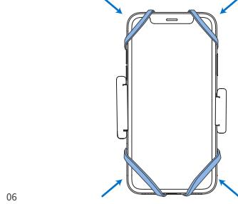
3. After use, remove the straps at the four corners and pull up to remove the phone.
