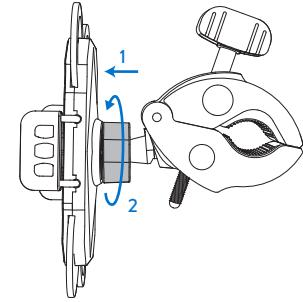
4. Loosen the adjusting screw and open the jaws of the bicycle fixed clip to the width of the handlebar.
