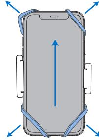
**Note:** This product comes with a spare silicone strap. If the silicone strap of the mobile phone clip is damaged after long-term use, please put the spare silicone strap on the round hole on the back of the mobile phone clip as shown in the figure, and then press the bracket. Installation steps can be used after installation.
